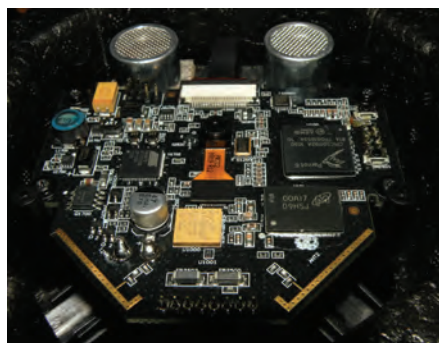
The main board is shown in situ; the two silver columns are the ultrasonic transducers that determine height above the ground
