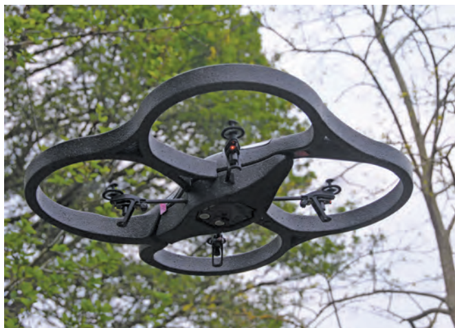
Looking from below you can see the transducers that control the height, this is with the Drone about 3 metres off the ground
