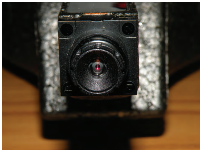
The front camera provides a wide-angle view which appears on the device you choose to use to control the drone
