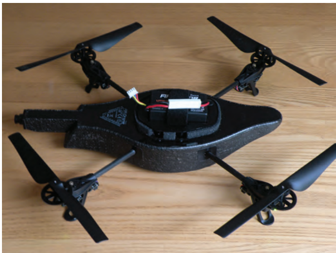
Here you can see the EPP hull that carries all of the electronics along with the battery in place
