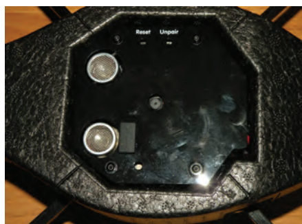
Below the Drone we see the camera in the centre, the USB port, the ultrasonic transducers with the reset and unpair buttons
