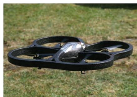
Flying in the garden with the EPP foam safety guard attached (TvG photo)
