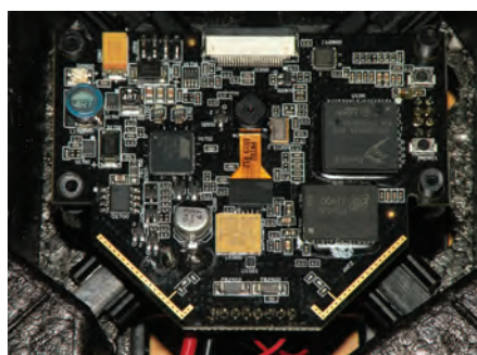
In the centre of this picture of the main board you can see the camera that looks underneath connected by the orange ribbon cable and the white connector is where the forward facing camera connects
