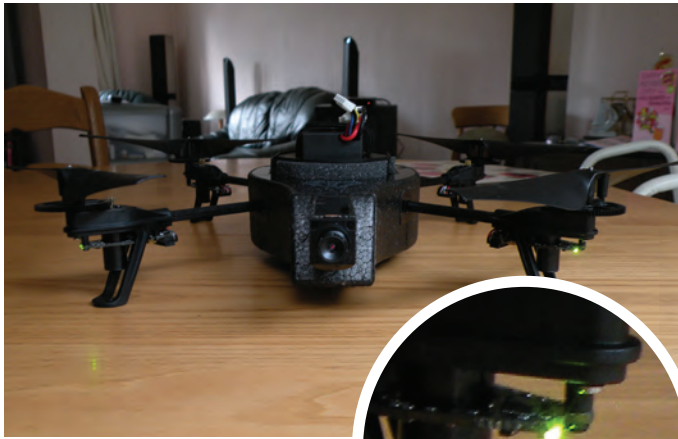
The green light indicates that the Drone is ready to connect to the control device
