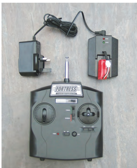
ABOVE LEFT: The Fortress has futuristic styling and a hard plastic shell protecting the front pod. ABOVE RIGHT: The business end of the Fortress - the robust fixed-pitch rotor head. FAR LEFT: The large coarse-pitch tail rotor is driven by a geared coreless motor. LEFT: The 27 MHz Tx of the Fortress - trims on yaw and pitch - and the charging system with UK plug/transformer, balance charger and 300mAh LiPo.
