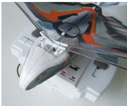
ABOVE LEFT: Charging the i-Bird on its controller - the double rocker mechanism and pushrods operating the wings are shown. ABOVE RIGHT: The i-Bird flaps its way towards the coving like a homesick angel. BELOW: The amazing Midland SpeedDome in Perth, WA, home of the newly formed Perth Indoor Flyers and venue for the first test flights of the two breeds of ornithopter reviewed here.
