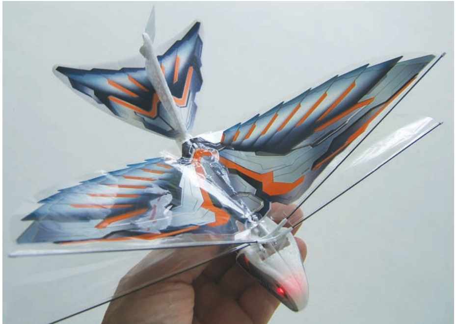
This shot shows the four-wing arrangement of the Wingsmaster series and a fully-deflected rudder.
