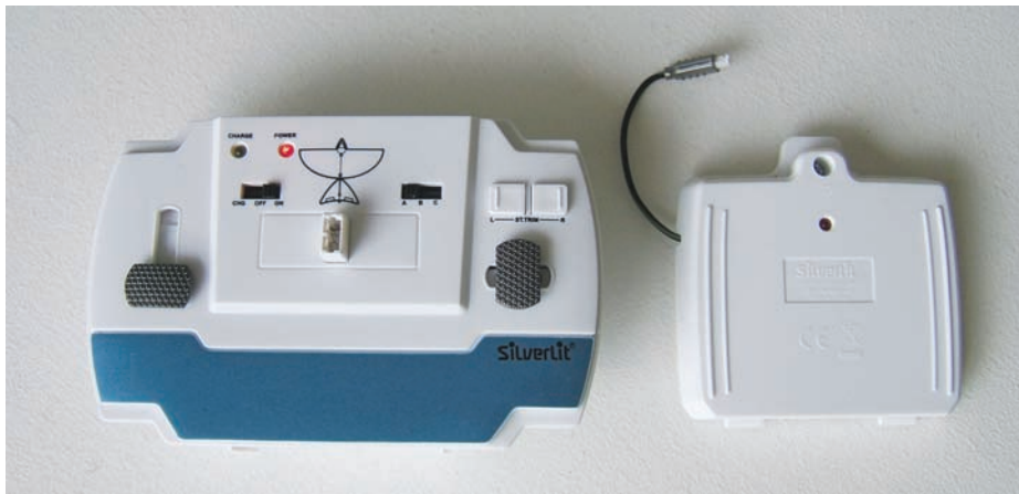
ABOVE LEFT: The Wingsmaster infrared controller, together with the £4.99 IR booster available separately. ABOVE RIGHT: The business-end of the controller with the IR booster attached, showing four extra LEDs.
