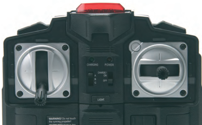
The 3-channel infra red Transmitter for the 'go forward' helis have forward speed buttons on either side of the Tx top.
