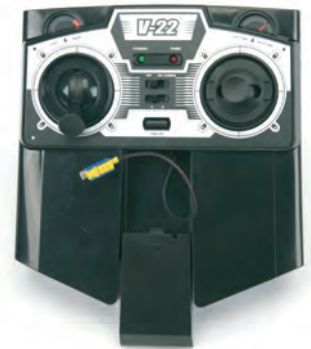
The Tx for the V22 VTO has a special 'take off button, that converts floor level motion into vertical hovering flight!
