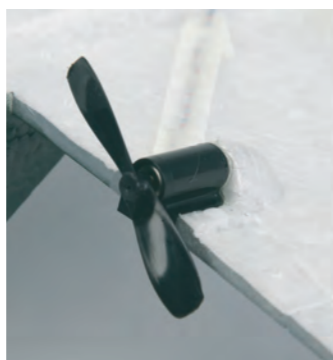
The twin motors have thrustlines built in.
