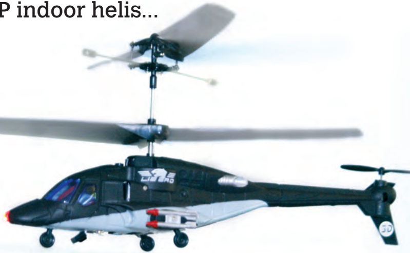
The Jamara Airwolf micro EP heli - contra rotating blades, horizontal tail rotor - and a hard bodysell. One of the next generation of this type of micro machine?
