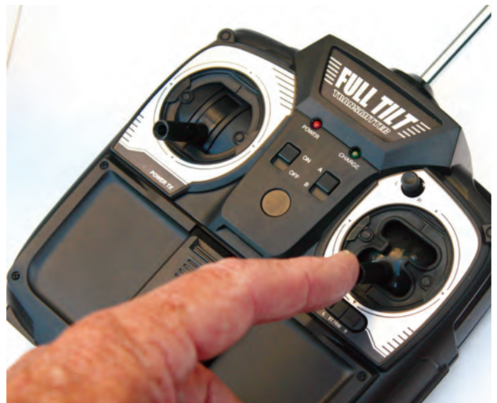
The right-hand stick operates transition and yaw
