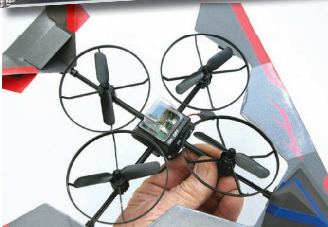
No assembly is required so this model is ready for action. Note the module in the centre of the lift motors and lightweight structure
