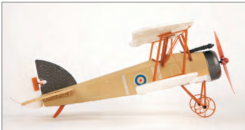
Denoted as proportional, in reality the rudder is of the 'all or nothing' variety.
