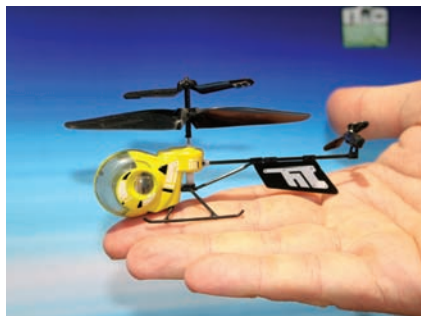
The Silverlit 'Atom' is one of the smallest and lightest infrared micro helis at 112.5 mm long and weighs just 8 g; can be conveniently stored in its own transmitter case
