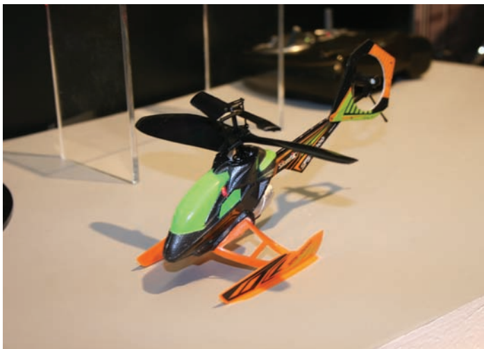
Silverlit's Picoo Z 'Air Slide' is a 3-channel micro heli and will make a smooth sliding lift off from a smooth surface
