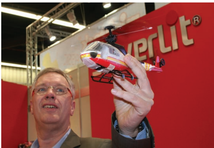
Designer of the Silverlit Picoo Z range, Alexander van de Rostyne holds the prototype 3-channel double-size Picoo Z-XL 'Vortex' ready for flight; the model features a Piezo Gyro System for stability indoors and outdoors in calm conditions
