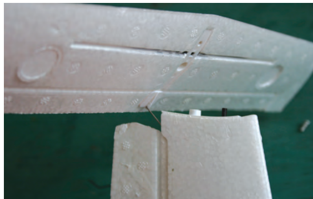
The stabiliser fits onto the fin with this plastic fitting and is held in place with a screw
