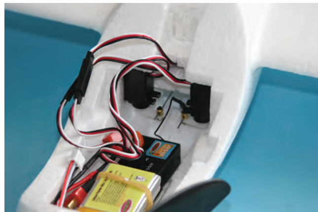
Elevator and rudder servos mounted to the rear of the cockpit
