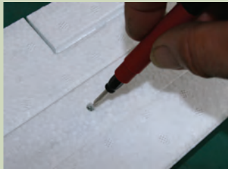
Be sure to tighten the wing retaining screw
