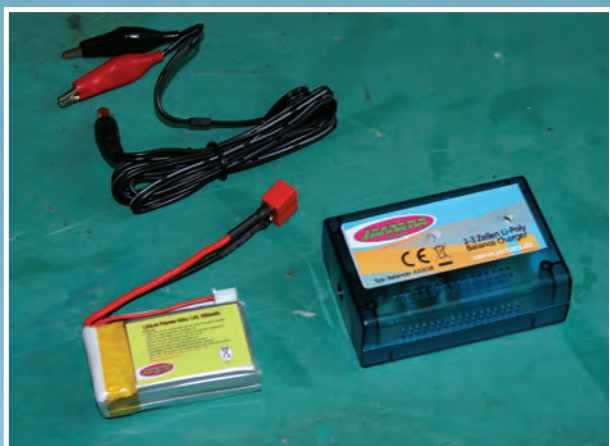
ABOVE: 1000 mAh 2s LiPo battery and balance charger supplied
