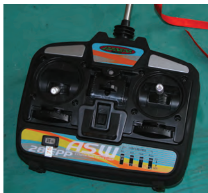
LEFT: This simple 35 MHz 4-channel transmitter comes with servo-reversing switches
