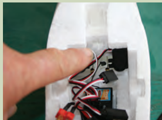
The two servo leads exit into the cockpit through this small hole and connect to a Y-lead
