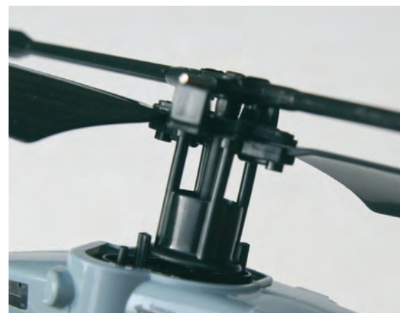
The rotor head uses the proven magnetic actuator system on the swashplate
