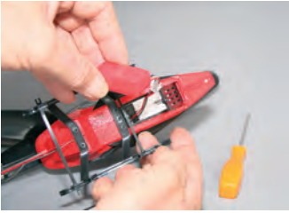
The 7.4 V 300 mAh LiPo is secured in the battery compartment
