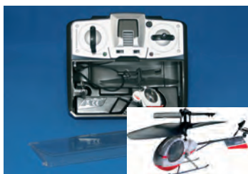
This tiny 9 g helicopter fits inside the transmitter and is used as a protective carry case
