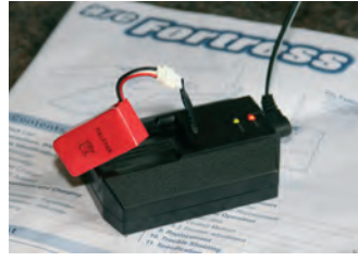
A mains battery charger is supplied for the 7.4 V 300 mAh LiPo
