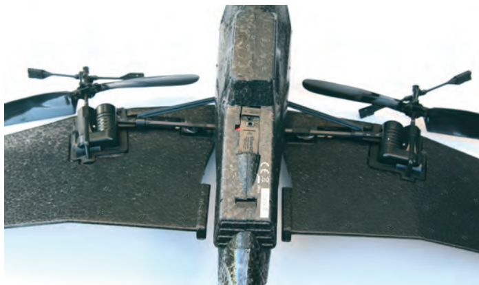
Motors and the wing rotating control rods
