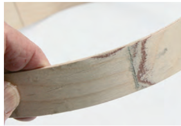
The double layer of 1 mm ply with the feathered joint
