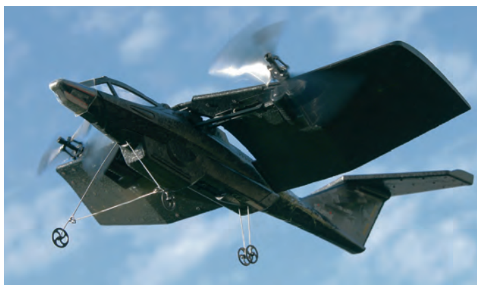
In aircraft mode the wing is still at a surprisingly steep angle
