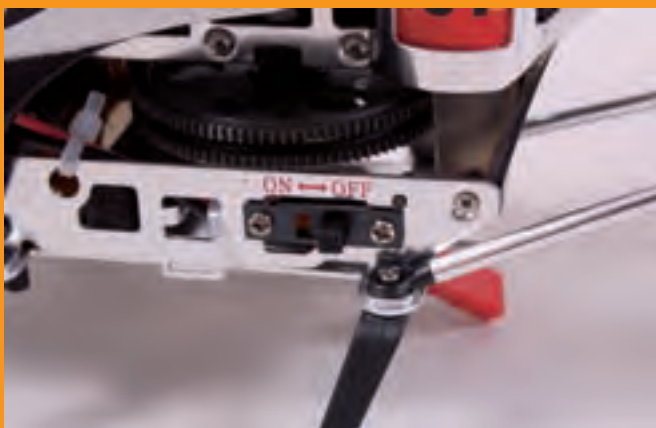
Having a 'proper' on/off switch helps when getting ready for a flight and acts as a handy reset for the electronics after a heavy landing or crash
