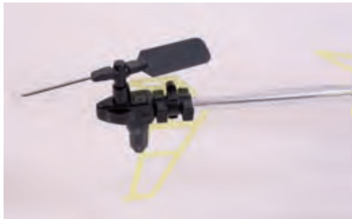
The small horizontally mounted tail rotor is used to give the Alutec its forwards and backwards movement and only operates when required
