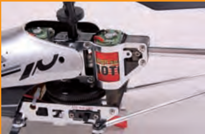
The Alutec is powered by a tiny electric motor and a 3.7V 1,000mAh LiPo battery pack that gives the model up to 10 minutes of flight time
