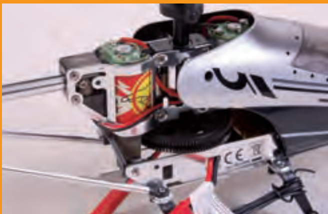
The use of lots of aluminium in the Alutec's construction gives it a good quality look and feel and adds to the model's rigidity and strength
