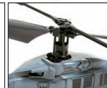
The head features a standard Silverlit fixed pitch single rotor and flybar
