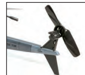
The powered tail rotor helps to steer and stabilise the model in flight
