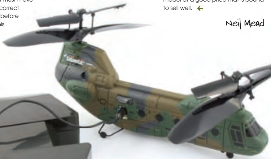
As with many of the other Picoo Z models, the Tandem is charged from the transmitter via a flylead. This can be tucked away inside the transmitter when not in use
