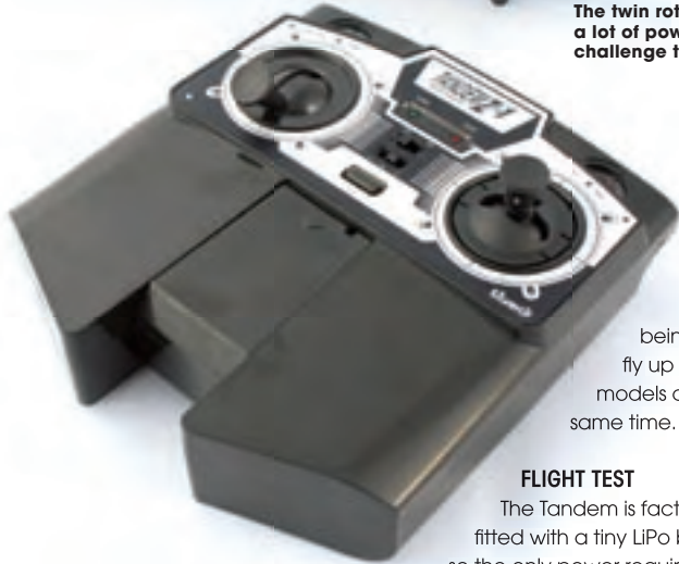
The infrared transmitter has a training plate fitted to the right-hand stick. This can be removed for full control
