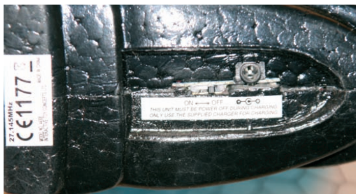
The charging point on the Vamp is in its belly next to the on/off switch.
