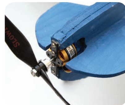
The Viper needed a different mounting to suit the Axi motor
