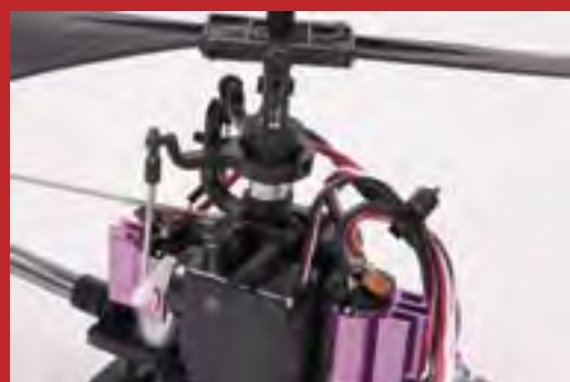
The servos control a simple rotor head arrangement
