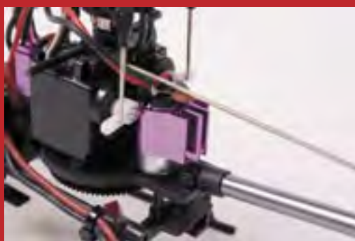
The tiny motors are quite powerful and fitted with heatsinks
