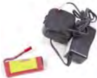
The 7.4V 500mAh LiPo and 240V mains charger
