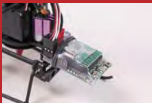
The electronic control unit sits at the front of the model
