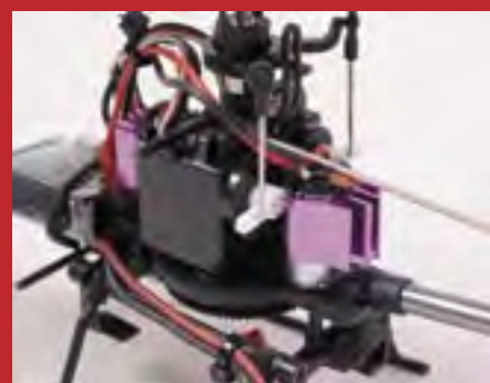
The Piwi is fitted with 'proper' mini servos
