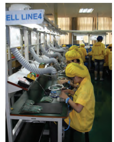
Circuit boards are built and checked in a temperature and humidity controlled environment.
